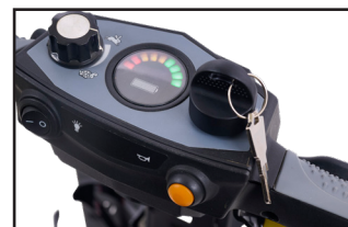
LED battery indicator on the console
