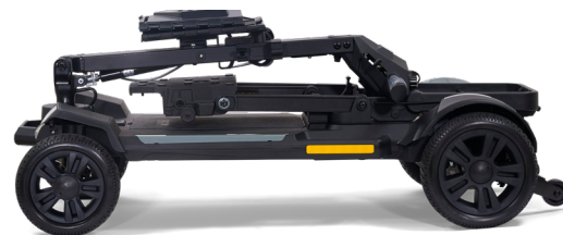
Folds easily for a compact profile of only 14" high (without seat)
